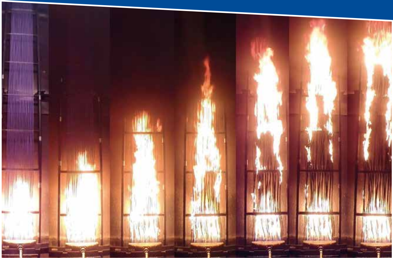
Figure 3 - Photo sequence showing the test progression of the cable shown in figs 1 and 2 - Time scale from left to right is < 6mins
