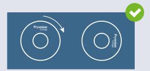
• When only a portion of the cable is used, the open end of the cable remaining on the drum should immediately be re-sealed to prevent the entrance of moisture. Once it has been resealed, the cut end should be fixed to the inside edge of the drum flange to prevent the end from extending beyond the flanges during drum movement.
