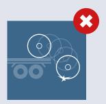
When using a fork-lift, the forks shall be long enough to support the full drum width. Always load the drum with the flanges perpendicular to the forks. Never support the drums with the forks placed between the two flanges directly on the cable. The distance between forks shall be enough to guarantee a stable position of the drum.
