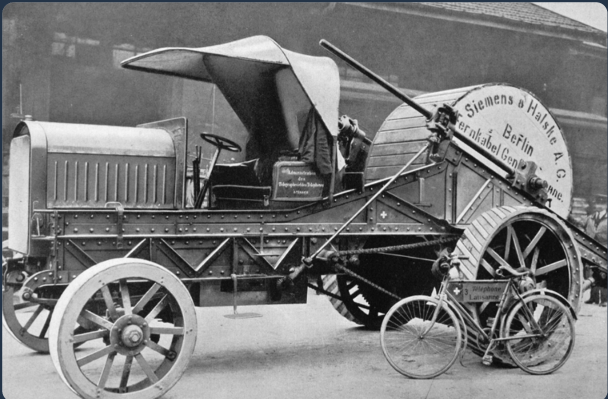
Cable transport wagon for laying telecommunications cable on the Geneva - Lausanne route, around 1920
